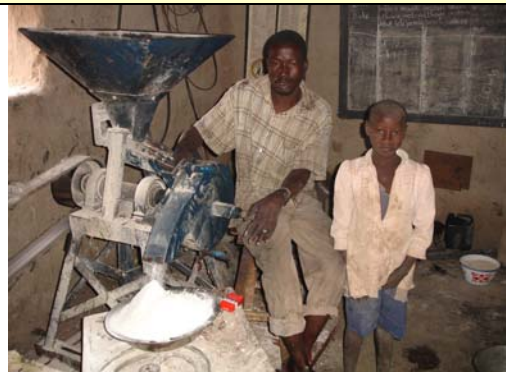
Milling flour in the grain mill of the women of M'Pegneso village, Sikasso Region, Mali. The mill grinds sorghum, rice and maize grains into flour.
